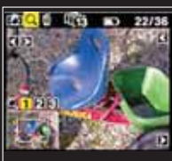
Magnification: Images can be magnified in Playback mode up to a factor of 1:1 in much the same way as most digital cameras do this. There are only three zoom steps, but the system works well enough. It is also possible to scroll around the zoomed image in order to check sharpness and the like.
